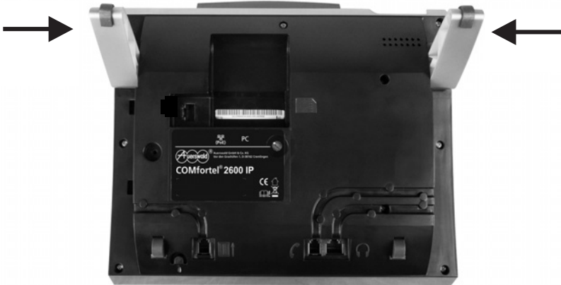
Fig. 8: Feet of the casing
