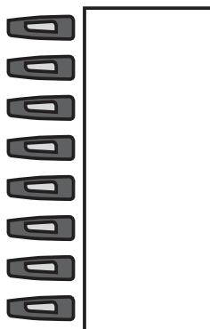
The **function keys** next to the lettering label are programmable keys, e.g. to assign speed dial numbers or operate telephone functions. Each key has two levels that can be assigned functions.
