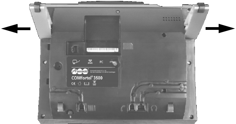
Fig. 6: Removing the feet of the casing
