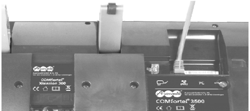
Fig. 10: Connecting the patch cable (here for the operation with Power over Ethernet)
