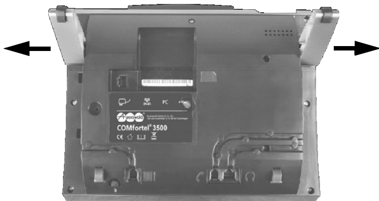
Fig. 6: Removing the feet of the casing
