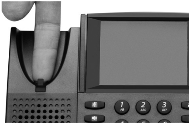
Fig. 12: Pressing down the insert
