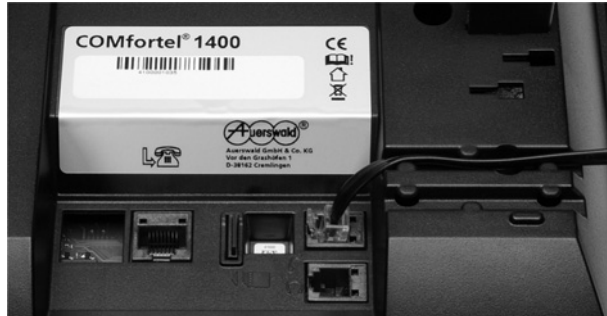
Fig. 13: Connecting the receiver
