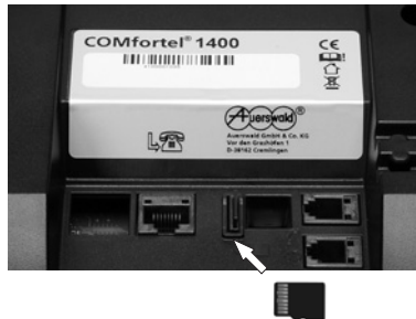
Fig. 16: Inserting the memory card
