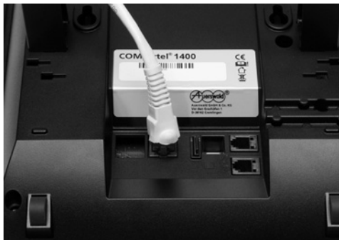
Fig. 15: Connecting to the PBX
